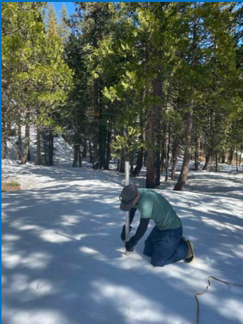
An NID hydrographer measures the snowpack at Bowman Reservoir in late March.
