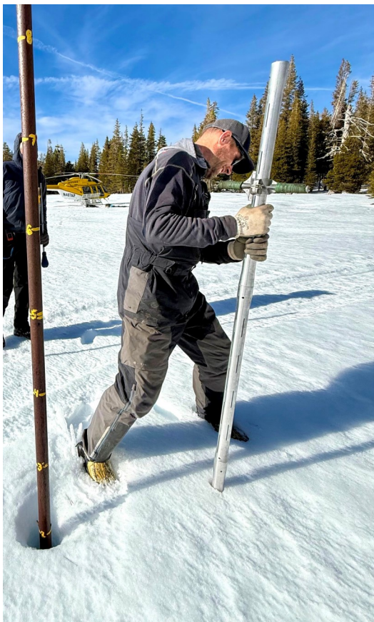
Above: an NID surveyor measures snowpack using a sampling tube at the English Mountain snow course.
