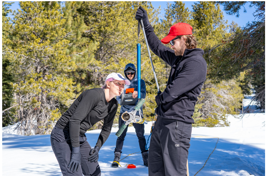
NID hydrographers conduct a snow survey on Findley Peak. Story on Page 3 .
