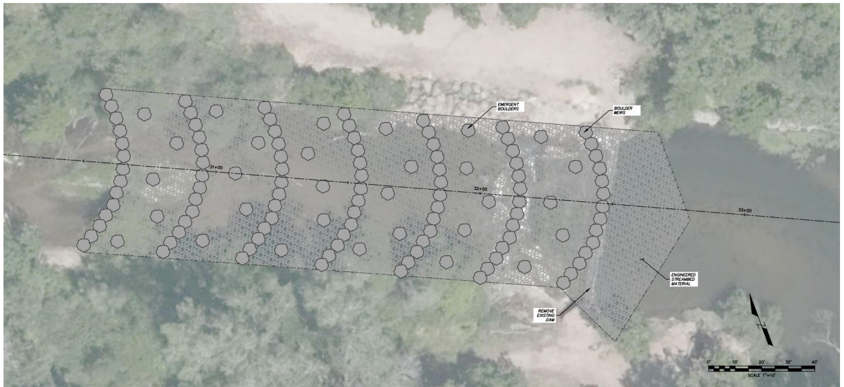
Figure 3-3. Profile and plan view of proposed roughened rock ramp (Alternative 2)
