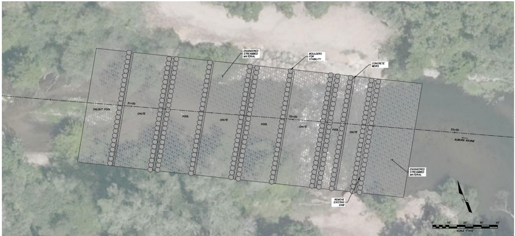
Figure 3-2. Profile and plan view of proposed chute and pool nature-like fishway (Alternative 1)
