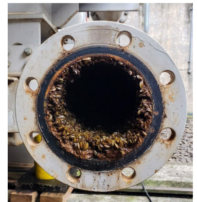
Golden mussels colonize a water pipe at a hydroelectric plant in Brazil in 2021.
