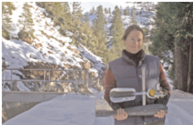
Hydrographer Jessica Erickson shows the velocity meter she uses to track flows. She is pictured along the Bowman-SpaULDing Canal near Fuller Lake.
