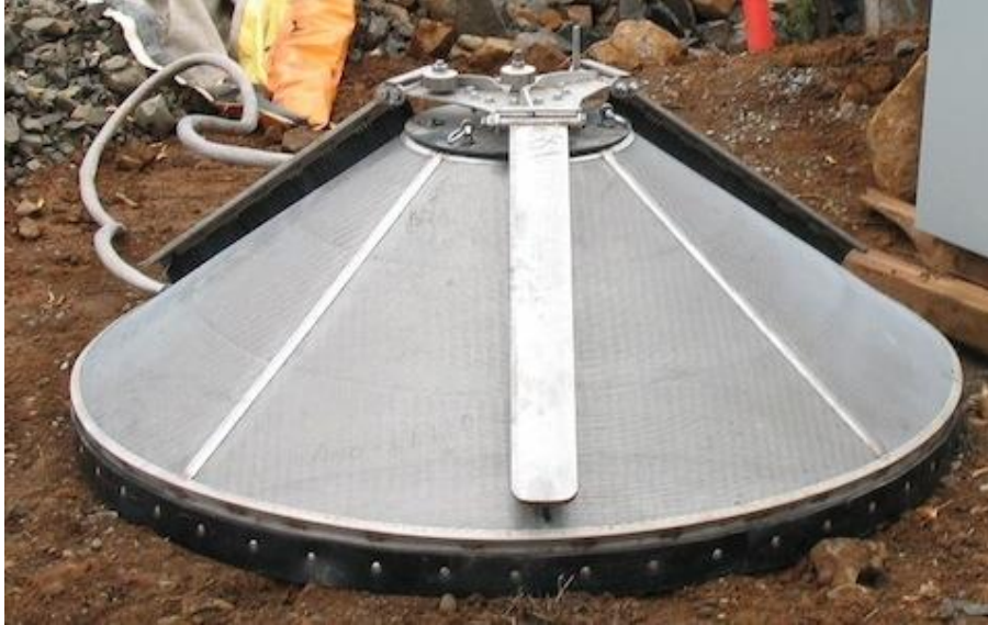
Figure 3-3. Cone Screen with External Brushes
